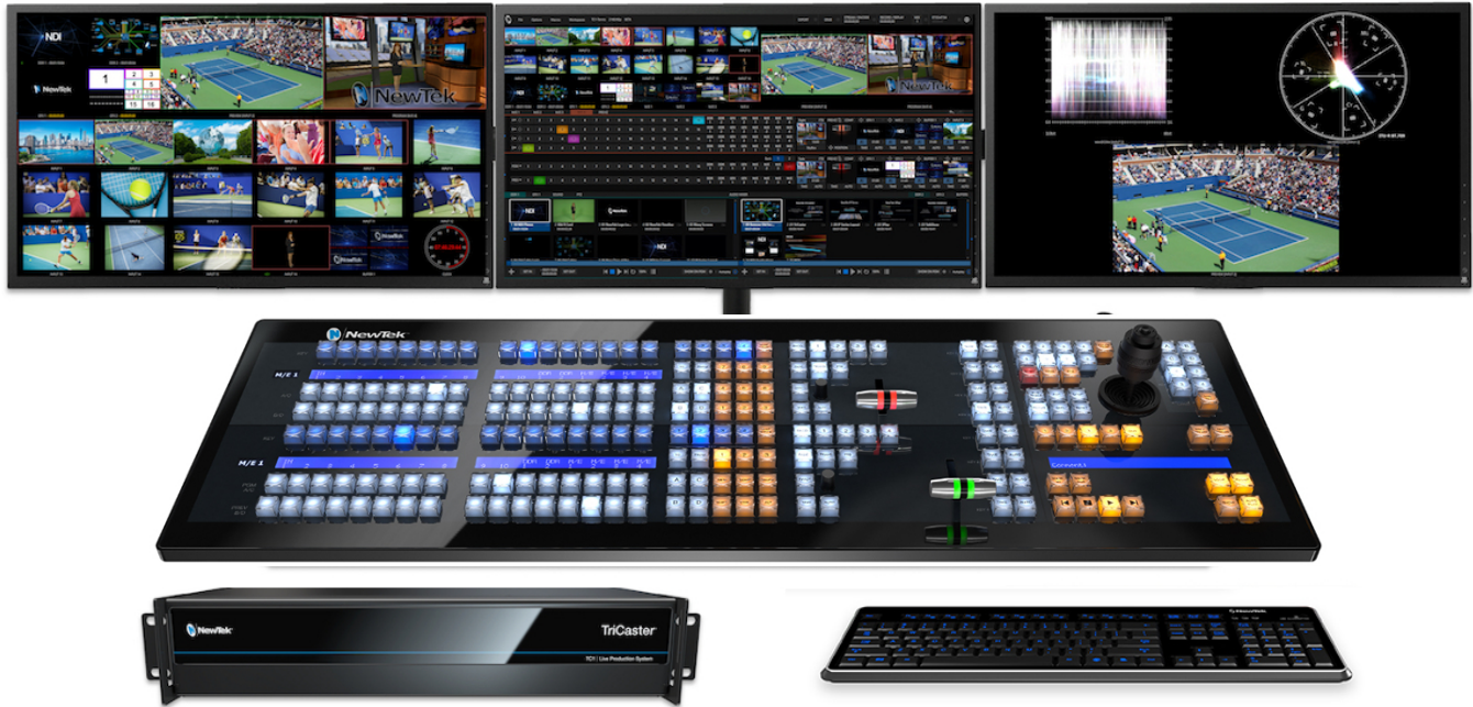
TriCaster TC1 live production system with TriCaster VMC 2S control panel
